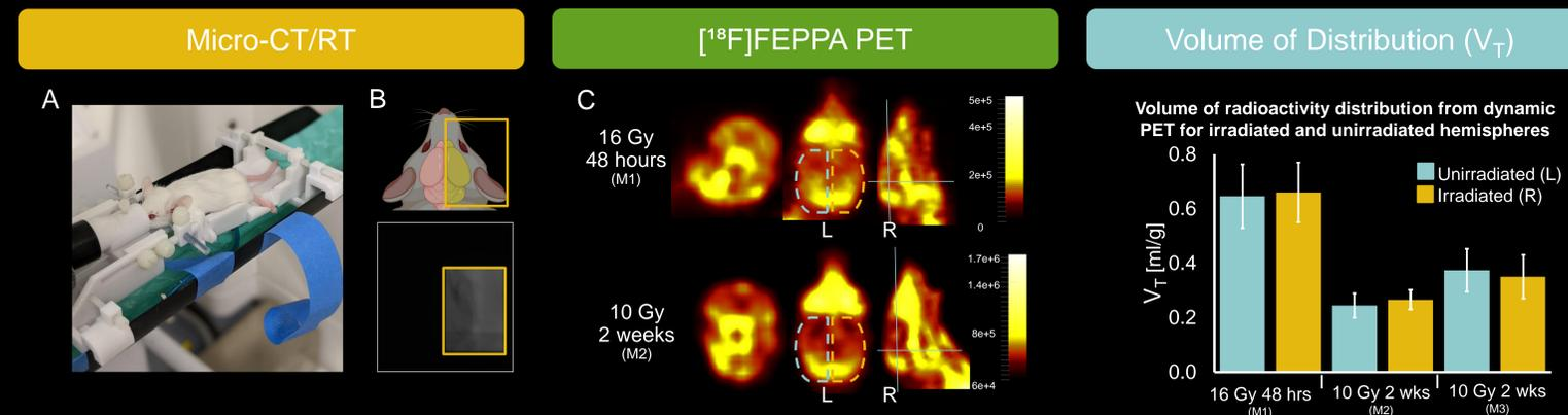
Figure 1. Diagrams and images for half-brain irradiation. A) Mouse setup on 3D printed animal holder on micro-CT bed prior to imaging. B) Diagram (top) and x-ray image (bottom) taken with micro-CT showing the irradiated hemisphere. C) Normalized [<sup>18</sup>F]-FEPPA PET [Bq/cc] images averaged over last 15 minutes of 90 minute dynamic PET scan for mice receiving half brain irradiation; representative ROI drawn to show the irradiated (yellow) and non-irradiated (blue) brain hemispheres.
