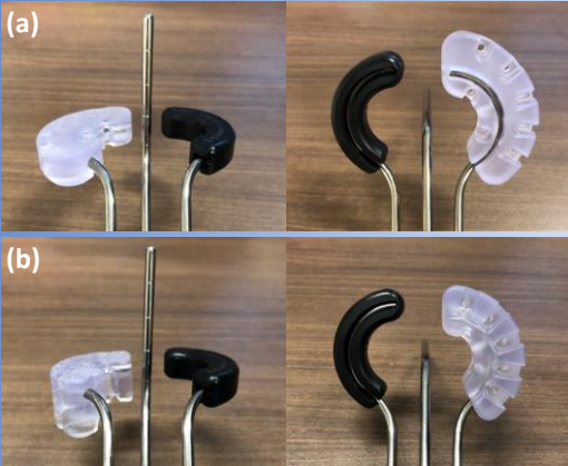
Figure 1. 3D-printed (a) M1 cap; (b) M2 cap assembled on the right SR of the CT/MR split-ring applicator and compared to the 5x5 build-up cap shown on the left SR.
