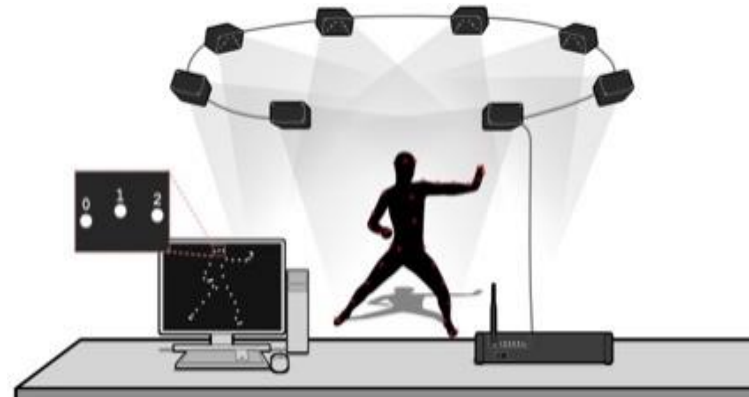
Figure 2: General setup of marker-based optical cameras for motion capture studies.
